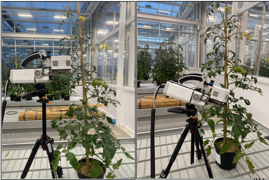
Figure 8. Li-6800 measurements of the higher leaf layer (left) and lower leaf layer (right) in compartment 3.
