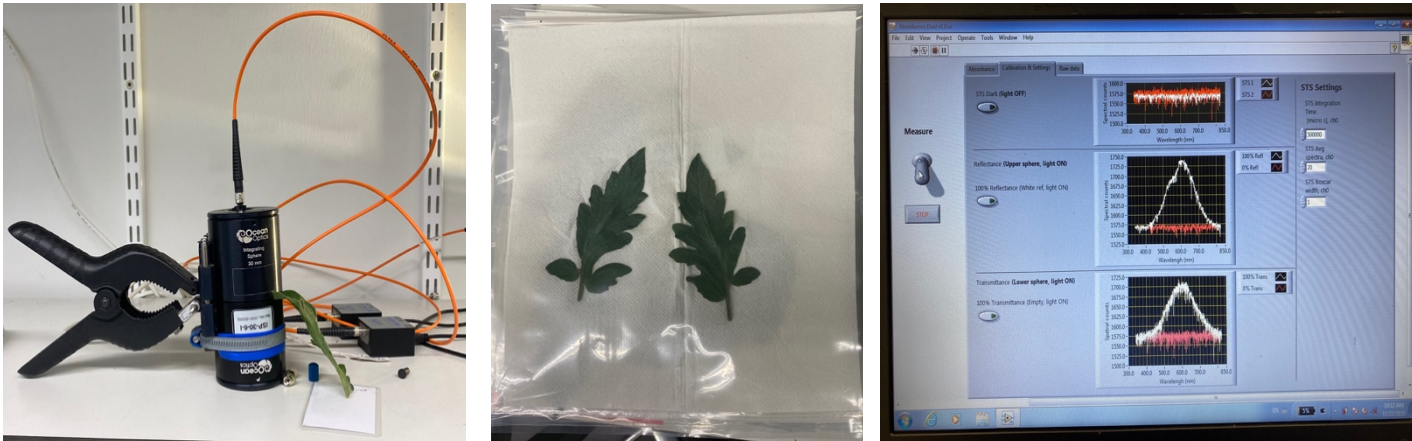
Figure 7. The two spectrometers (A), the leaflets as stored in plastic sheets (B) and the measurement software (C).
