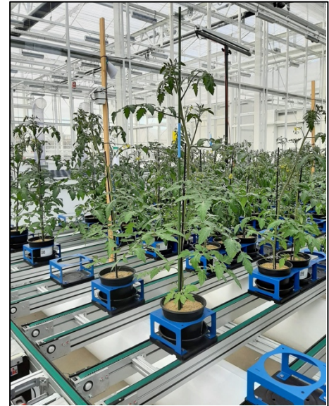
Figure 4. Showing the tomato plants in single carrier conveyor belts placed in the 23 cm pots with the growth sticks.
